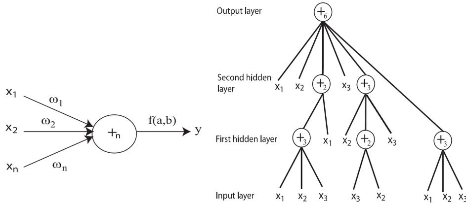
Fig. 1. A flexible neuron operator (left), and a typical representation of the FNT with function instruction set  $F = \{+2, +3, +4, +5, +6\}$ , and terminal instruction set  $T = \{x_1, x_2, x_3\}$  (right).
